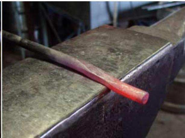
Take a heat (about 80mm) on the end of the bar and set it on the anvil with around 40mm protruding over the front edge. Using half blows, forge a shoulder on one side of the bar to about half the original thickness of the bar. Where the narrow neck is formed, this is the start of the leaf stem.
