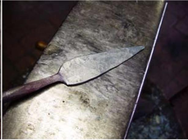
Carefully heat the tapered section (without burning the tip off) and forging on the anvil, flatten the entire length on the face of the anvil to a nice slender gum leaf shape. Refine the shape on edge if required.
