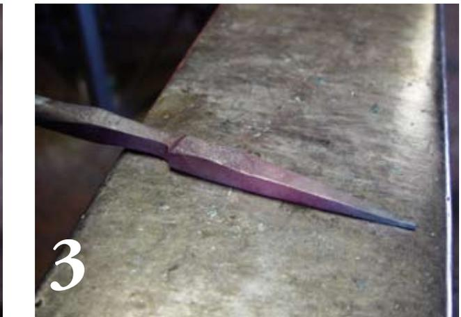
Rotate the bar 90 deg. (either direction) without moving it forwards or backwards and forge a shoulder as per step 1. Rotate back and true up the shoulder. Be careful not to thin the stem too much at this stage. You should now have an offset shoulder on two sides only, with a 12 x 40mm block on the end of the bar.
